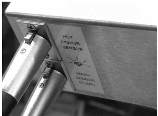
Step 3: Attach the short sensor cable to the hot liquor tank temp sensor (located below ball valve) (Figure 4). Align the indexing tabs on the cable and the sensor and push the connector onto the sensor. Note: to remove sensor cable, pull back on outer metal sleeve (never twist the sensor cable connectors)
