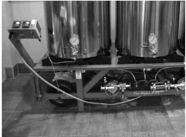
Step 1: Attach the digital control panel bracket to the left front upright of the brewery frame using the two included snap pins as shown (Figure 1)
