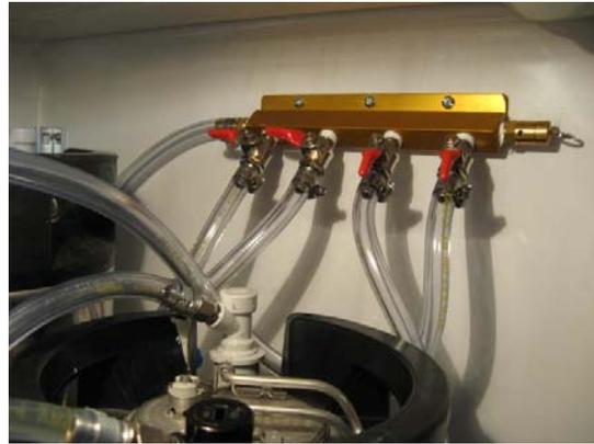
Determine where the "split" will be located, then measure from the outside regulator to the split for the first length of gas line. The rest will be 3-4 feet or 6 feet per your requirements.
